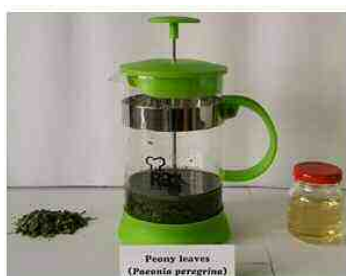
Fig. 2. “French press” type extractor used to prepare aqueous extract from peony leaves
