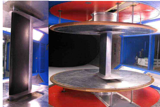
Figure 2. Visualisation of the Morphing Wing in the Wind Tunnel at the IAR-NRC
