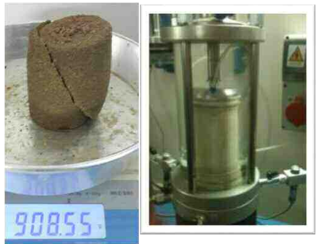
Fig. 2. Treated sand sample with the relative density 60% in the triaxial test cell (right), the sample after the failure (left)
