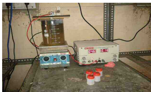
Fig (1). Batch electrochemical set-up
