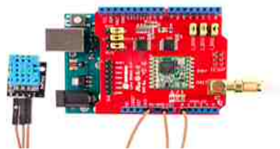
Fig. 4. DHT11 connection to the Dragino shield - top view
