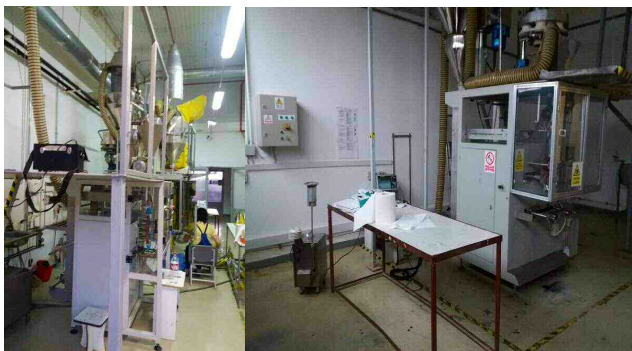
a) b) Fig. 2. Photos of the measurement campaigns for detecting particle concentration using the GRIMM dust monitor (a) in a technological production hall, and (b) a classic gravimetric instrument mounted in a packaging hall.
