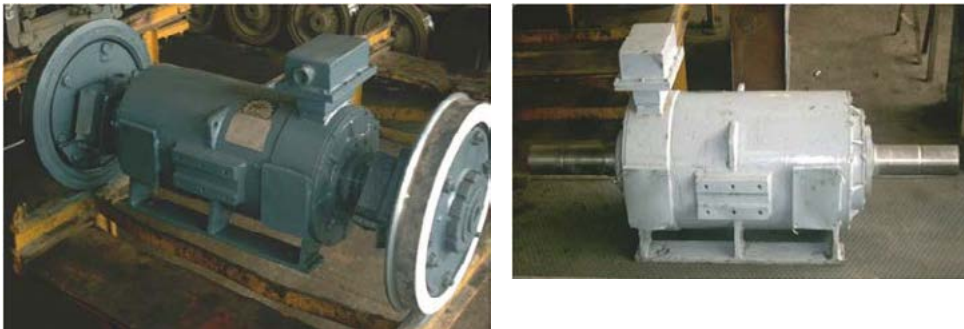
Fig. 2.27 The wheel-set fastened to the motor prototype.
