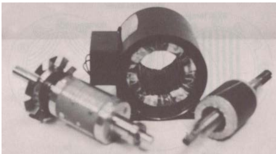
Fig. 14.4 1.5kW, 2pole, 3600rpm ALA rotor RSM prototype, after [1, 2].
