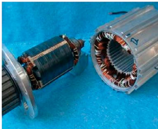
Fig. 14.16 The BEGA prototype: 1500W at 1500rpm, 2p = 4 poles.
