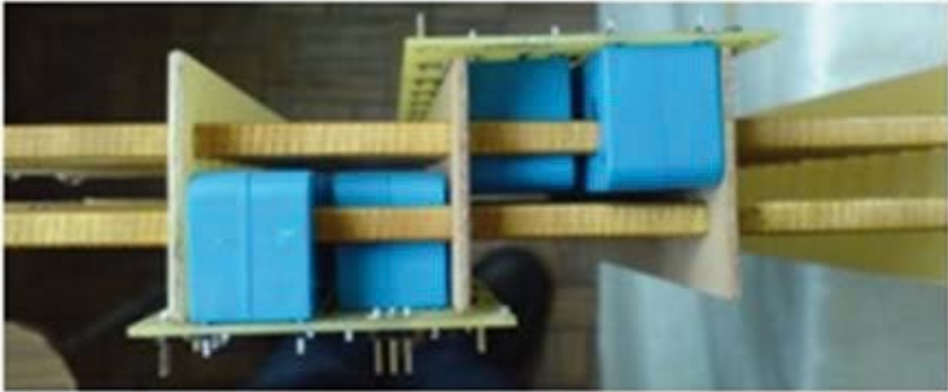
Fig. 2.16 Model bar with current transducers mounted on each subconductor.
