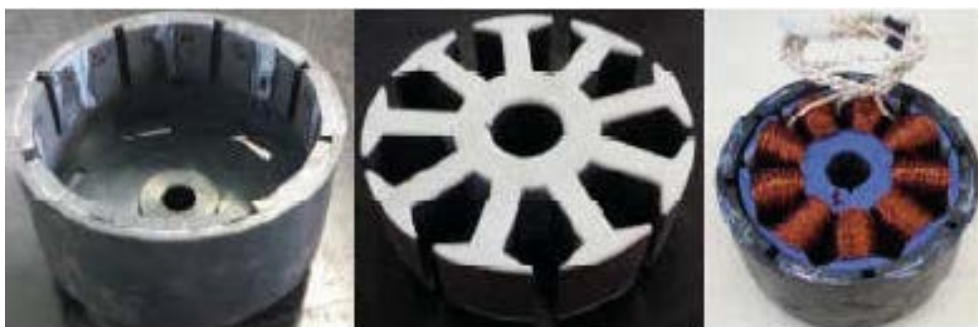
Fig. 8.24 The outer rotor PM motor prototype.
