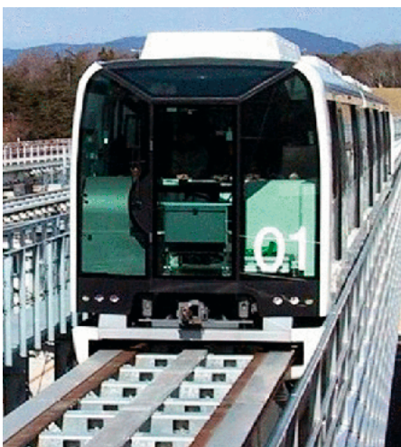
Fig. 12.2 Single-sided LIM-LINIMO-MAGLEV in Japan
