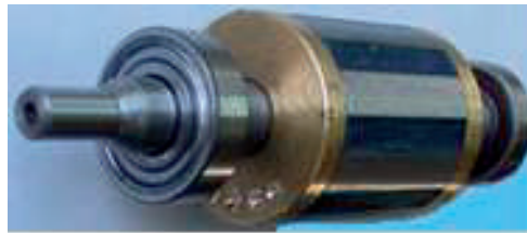
Fig. 7.21 The PM-RSM with the flux concentration rotor (PM-RSM-FC).
