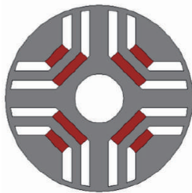
Fig. 7.1 Transversally laminated PM-RSM.
